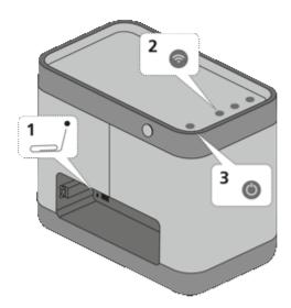
During reset, the On/Off and volume buttons flash. When completed, Beolit 12 switches to standby. Note that after a reset to factory settings, you must set up Beolit 12 again to connect it to a wireless network.
