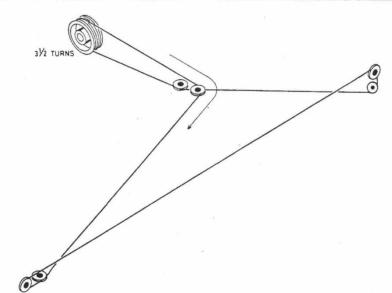
Dial cord is cut to a length of 125 cm and mounted as shown in the sketch.
